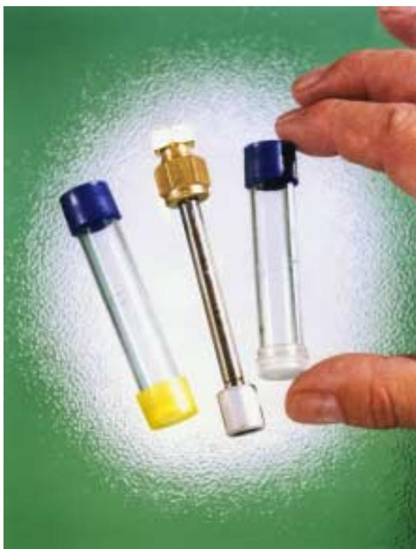
Figure 1: Diffusion tubes for (left to right) SO<sub>2</sub>, BTX and NO<sub>2</sub>
